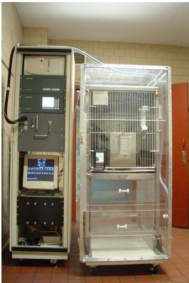
Figure 1 Monkey EMTAC showing the instrument rack to the left side of the Plexiglass enclosure. The Plexiglass enclosure is shown with the monkey metabolic cage and phantoms inside.
